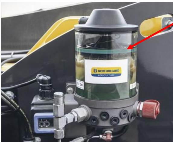
Pump with integrated control unit (1) , located on the left-hand side of the rear chassis
